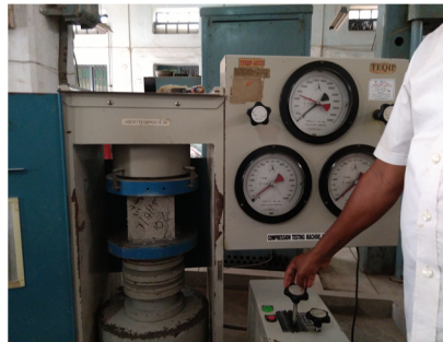
Fig 1. Test procedure of the SIFCON specimens
